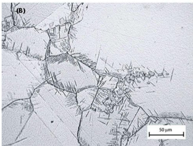
Figure A.8—Unacceptable Microstructure for UNS N07718 Showing Acicular Grain Boundary Precipitates; Original Magnification: 100X for Upper Photomicrograph (A); 500X for Lower Photomicrograph (B)
